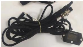
COM cable and Battery Meter
