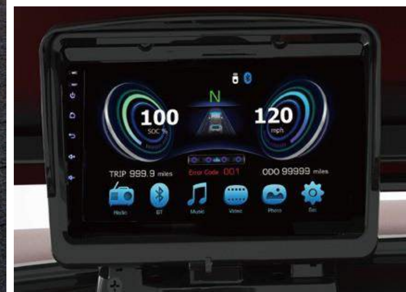
9" MULTI-FUNCTIONAL TOUCHSCREEN Touchscreen integrated with speed display, Driving Gear indication, Lights, Odometer, Radio, Music, Bluetooth Connection, Back-up camera image display., etc
